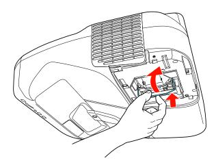
8. Tighten the screws to secure the lamp.
